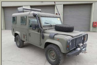
Land Rover 110 CAV 100 Enhanced Protected Vehicle , Land Rover Defender 110 is constructed of composite armour to defeat munitions up to 84 spec, 300 TD Diesel Engine, R380 Gearbox, Upgraded Heavy Duty Front Ventilated Disc Brakes & Rear Disc Brakes, Salisbury Front and Rear Axles Power Steering, etc, mileage from 58,000km, Excellent condition, Guide price from £25,000 (10 Available)
